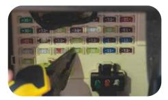
c. Install the fuse you just removed into the installation kit add-afuse circuit
