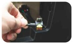
d. Plug the add-a-circuit into the fuse box in the correct orientation
